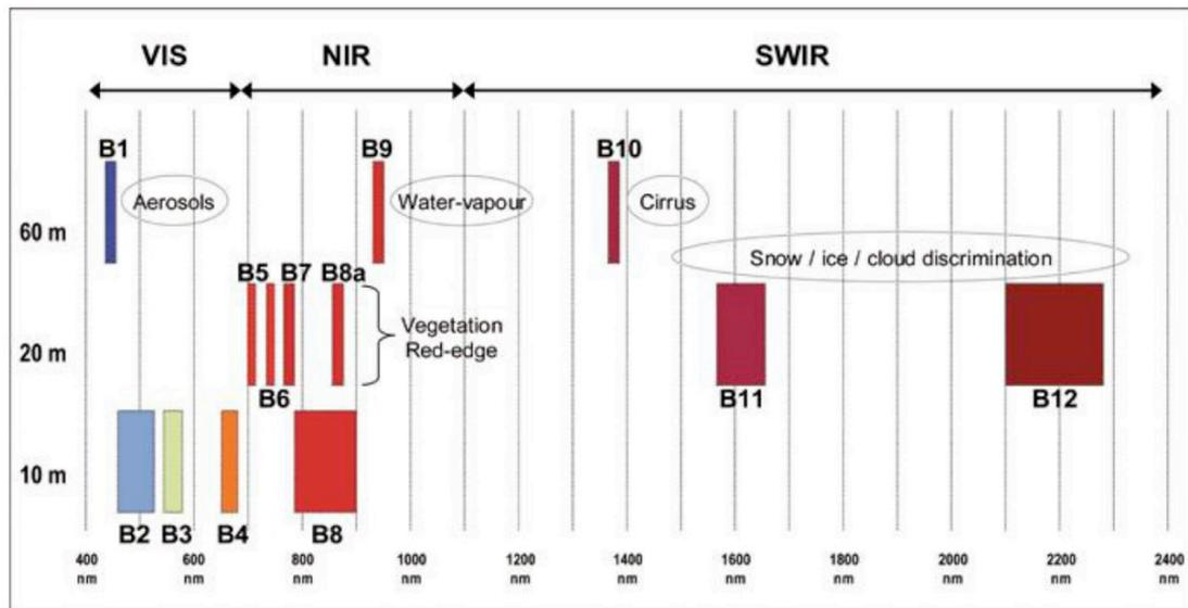
Fig. 2.2: Spectral range and spatial resolution of the 13 bands from the Sentinel 2a MSI sensors (Source: ESA SP-1322).
