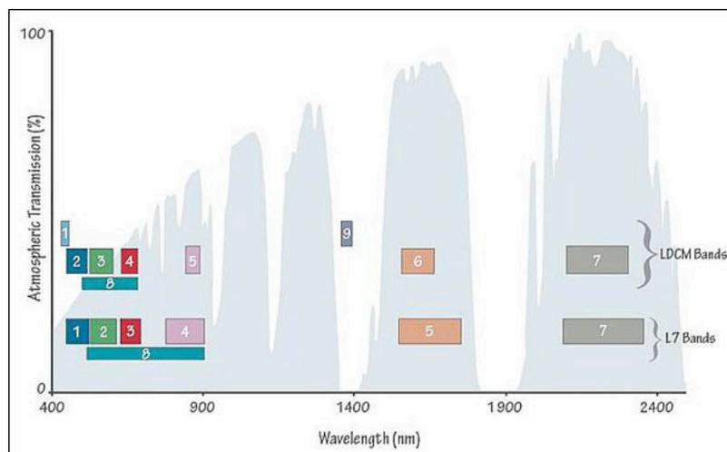
Fig. 2.1: Comparison of spectral bands from Landsat ETM+ and OLI (LDCM) sensors (Source: [http://www.csc.noaa.gov/digitalcoast/\\_img/Spectral\\_bands\\_of\\_landsat.jpg](http://www.csc.noaa.gov/digitalcoast/_img/Spectral_bands_of_landsat.jpg)).
