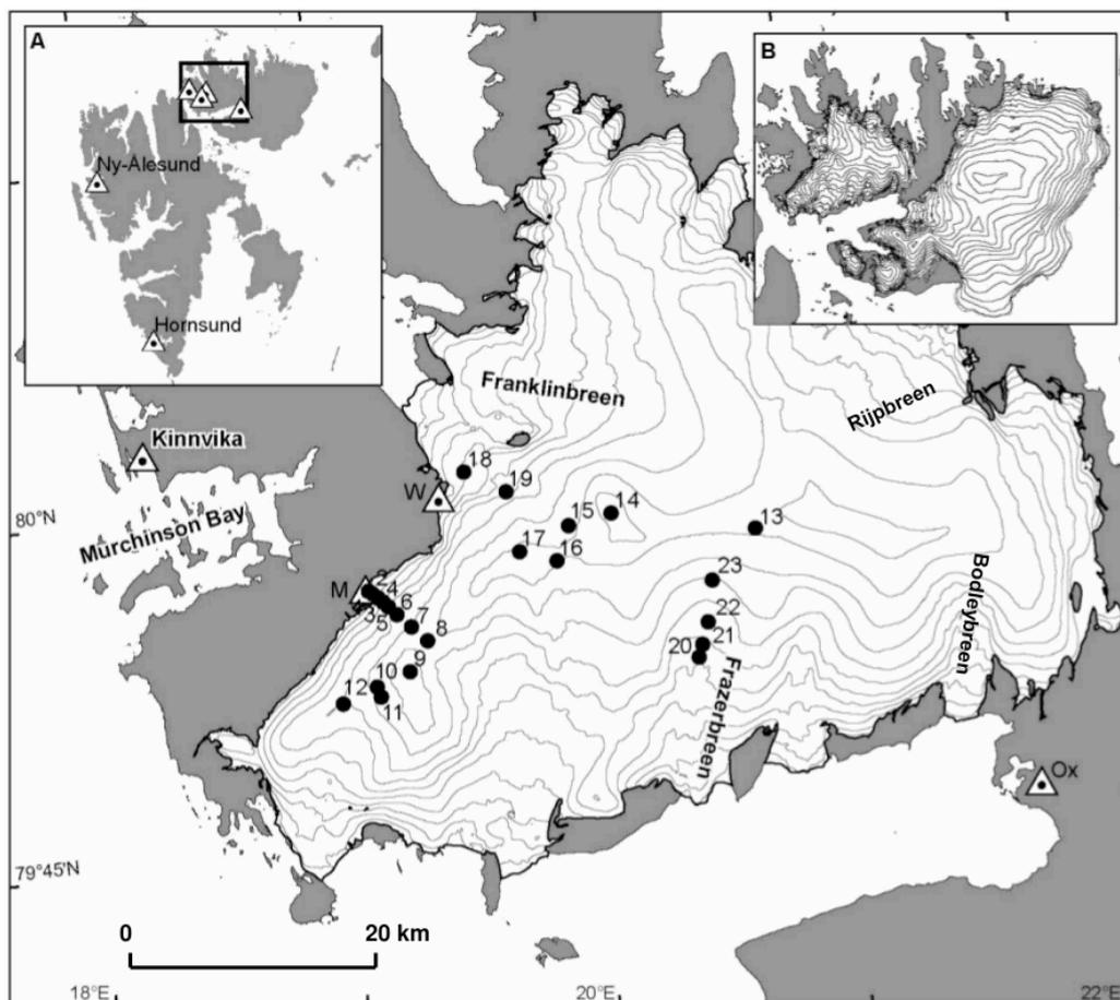
*Fig. 5.1: Svalbard, Nordausdlandet and the ice caps Vestfonna and Austfonna. Elevation- and coast line contours are from the Norwegian Polar Institute DEM. The elevation contour spacing is 50 m. The black dots mark the position markers used for DGPS surveys within the KINNVIKA project over Vestfonna. The triangular symbols are the fixed points / base stations, the letter at each fixed point / base station refers to the first letter of its name. Taken from Pohjola et al. (2011).*
