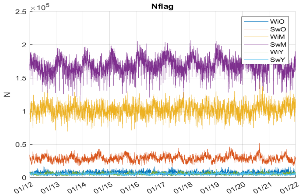
Figure 8: Number of flags raised as a function of time for the 6 L2OS classes from ERA5 model
