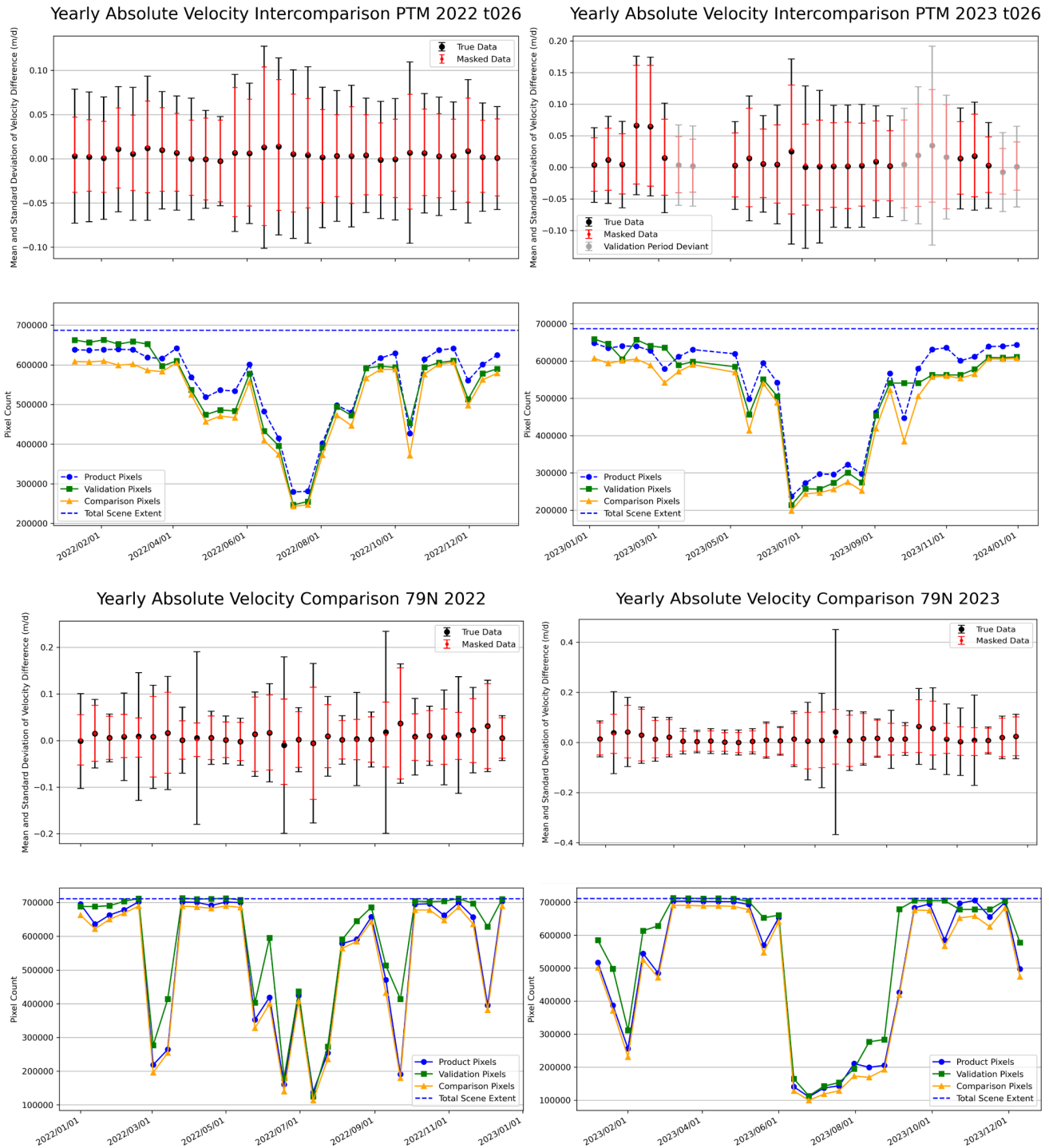
Figure 3-3 : Results of individual pair comparison for each location for two years. The upper plot shows the standard deviation of the velocity difference over each pair for both the masked and unmasked data. We have only included one of the tracks for the Petermann as they both show a very similar result. We therefore only include track 026 as it has better spatial coverage.
