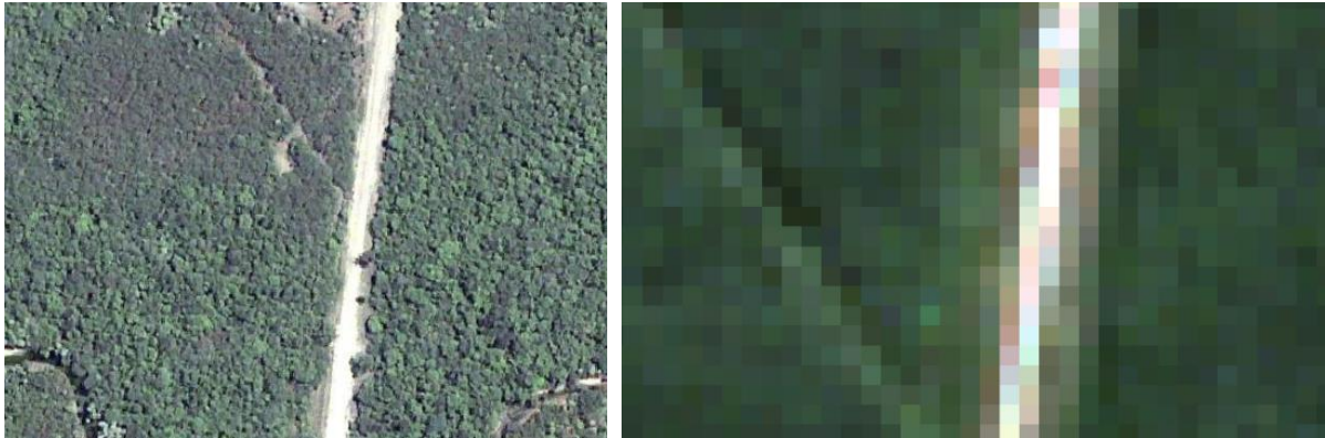
Figure 21. In Amazonia, the roads far away the city are not asphalted, and they are very similar to bare areas (ambiguous definition from the RS view point).
