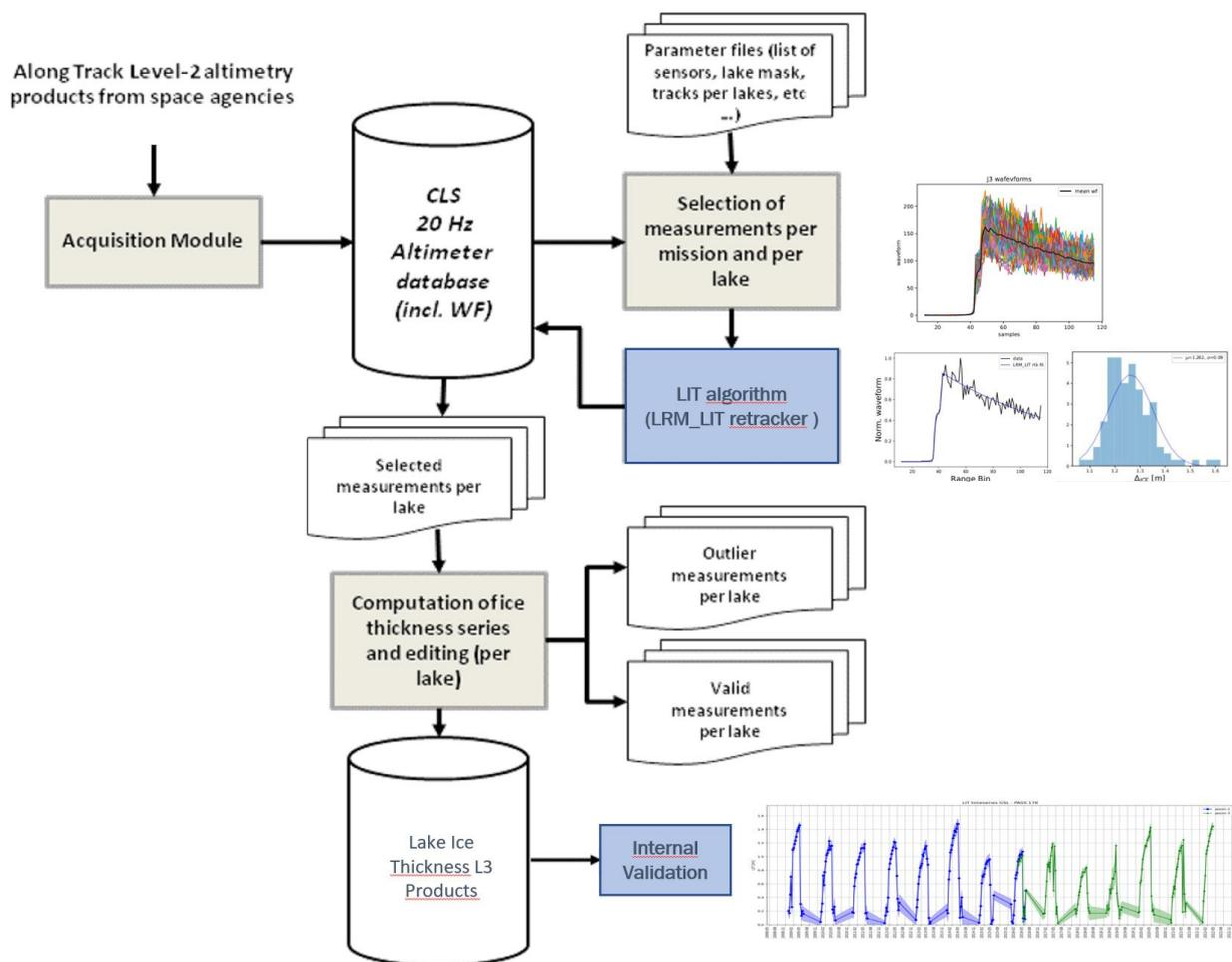
Figure 11. LIT processing system summary diagram
