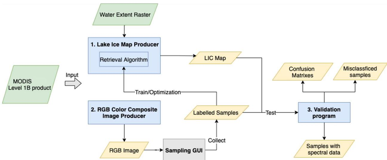
Figure 10. Overview of the LIC mapping system
