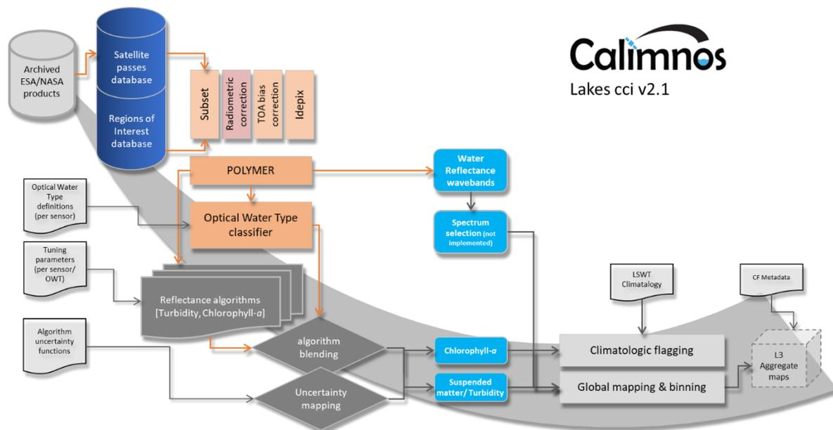
Figure 7: Schematic overview of the Calimnos processing chain for LWLR, Chlorophyll- $\alpha$  and turbidity or suspended matter.
