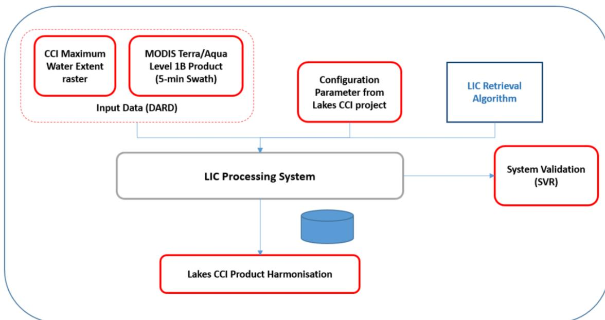
Figure 8. LIC Processing System: Context Diagram
