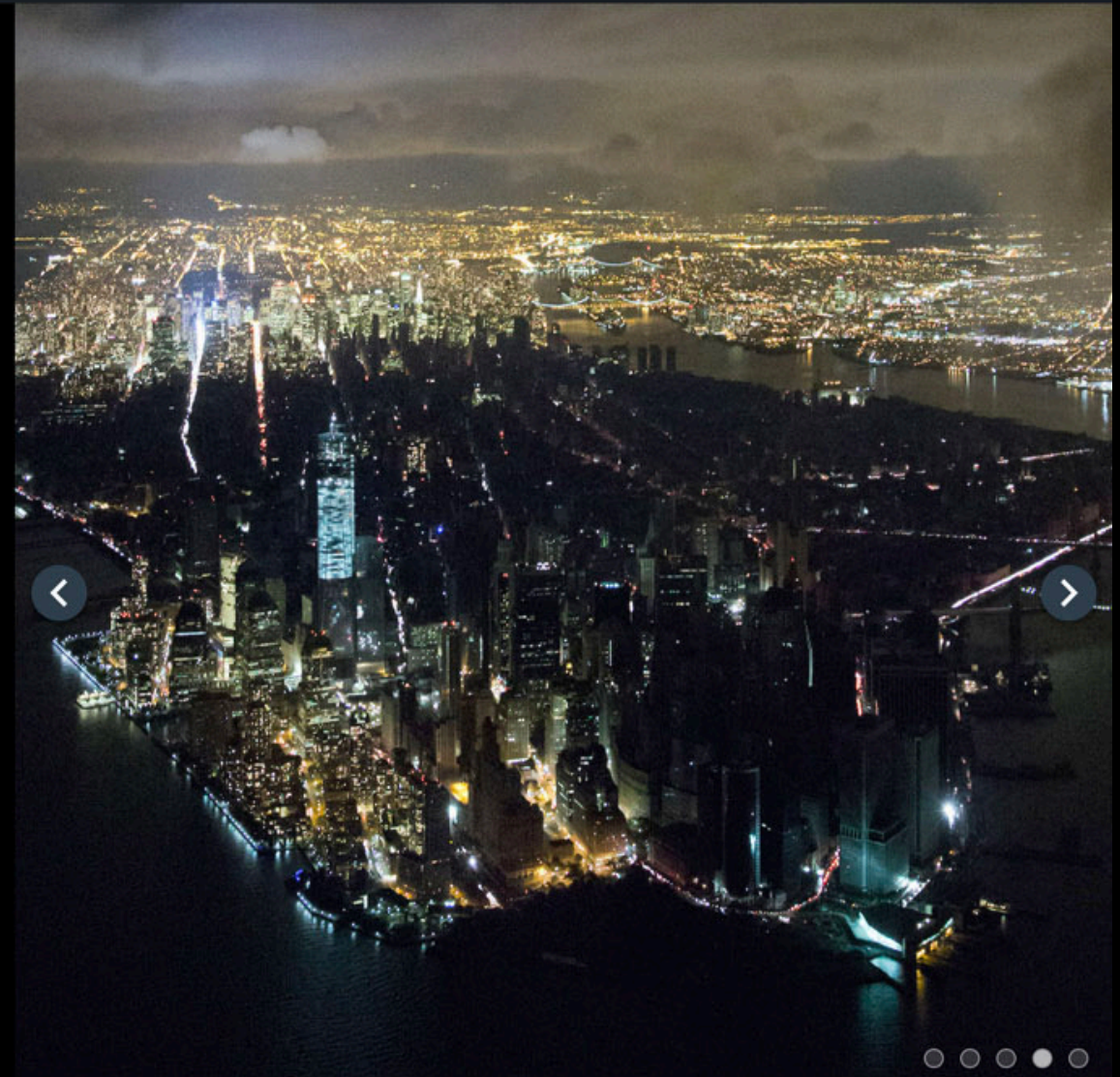
Blackout in New York after Hurricane Sandy, October 2012. The storm coincided with a "spring" high tide, resulting in a storm surge almost five metres above mean low water. Road tunnels, subways and electrical substations were flooded in lower Manhattan, and almost 2 million people were left without power across New York and New Jersey. (Iwan Baan/Getty Images)
