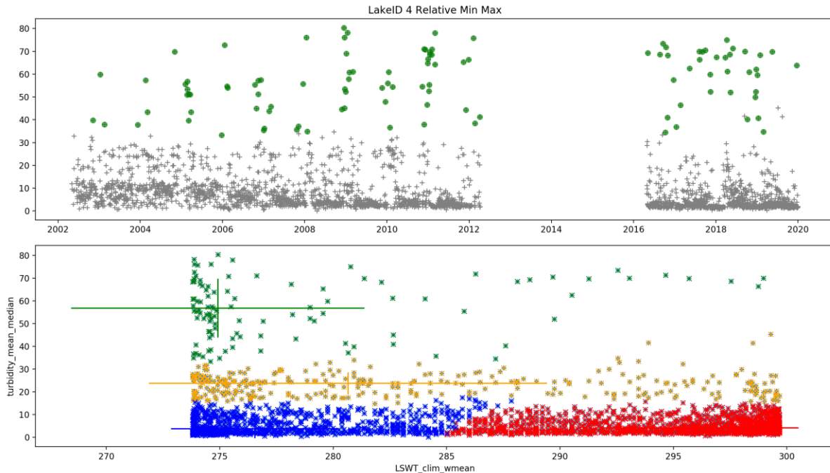
Figure 30 Turbidity time series and cluster analysis of daily lake-median turbidity and LSWT climatology. The green cluster, with its centre at low temperature and high turbidity values, is excluded because these data points are suspected to be undetected ice.
