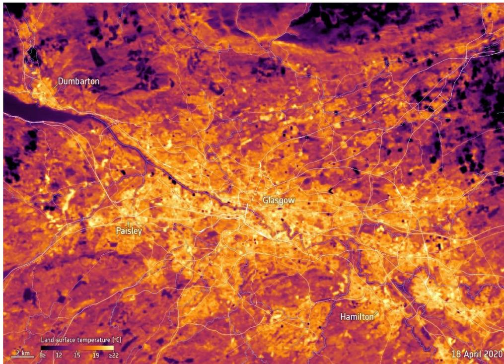
Figure 2: High resolution LST from LST\_cci for Glasgow, UK from Landsat-8 satellite for 18<sup>th</sup> April 2020. (Credit: LST\_cci, NCEO, Space4Climate for algorithm and data; ESA for visualisation)
