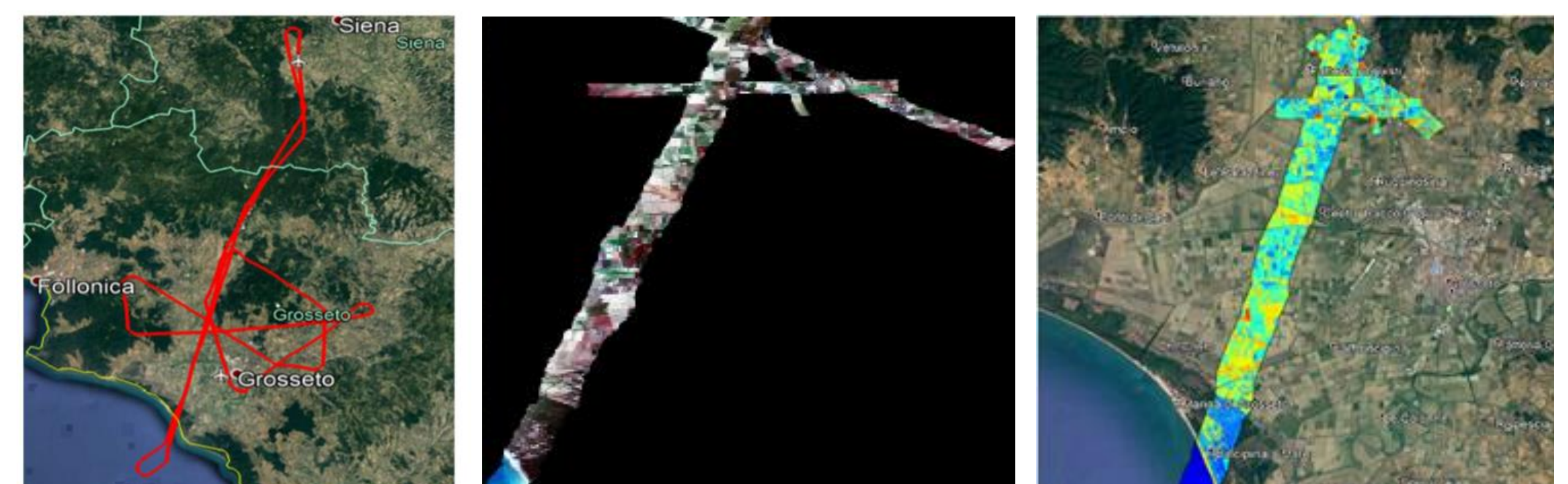
Fig 4: (i) Flight path over Grosseto, Italy (ii) L2 FENIX Reflectance (iii) L2 HyTES Land Surface Temperature
