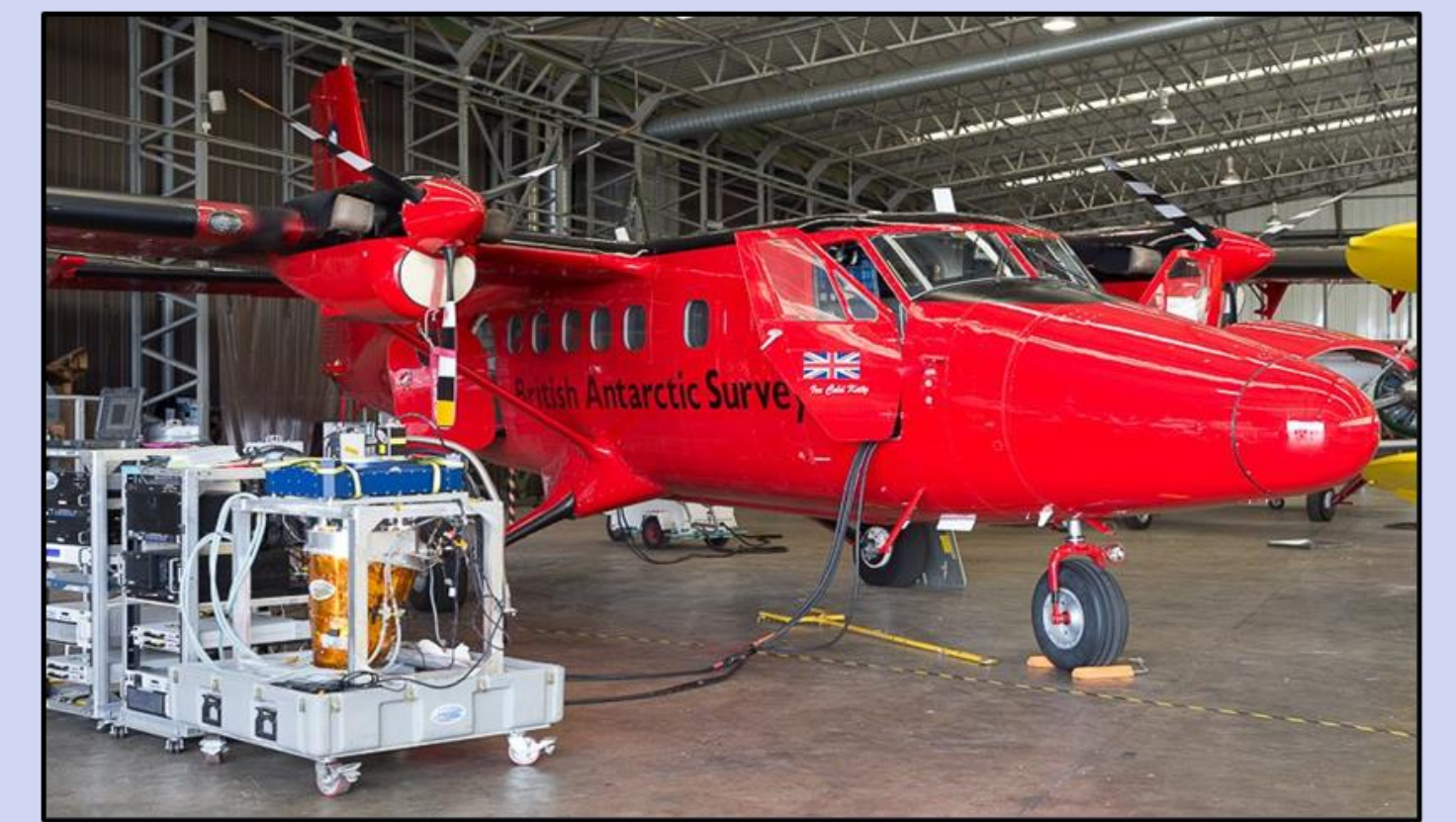
Fig. 1: HyTES sensor being installed into the British Antarctic Survey (BAS) Twin Otter Plane
